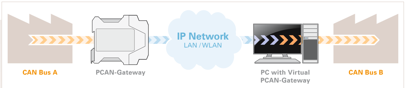
Example 4: Connection via the software Virtual PCAN-Gateway
