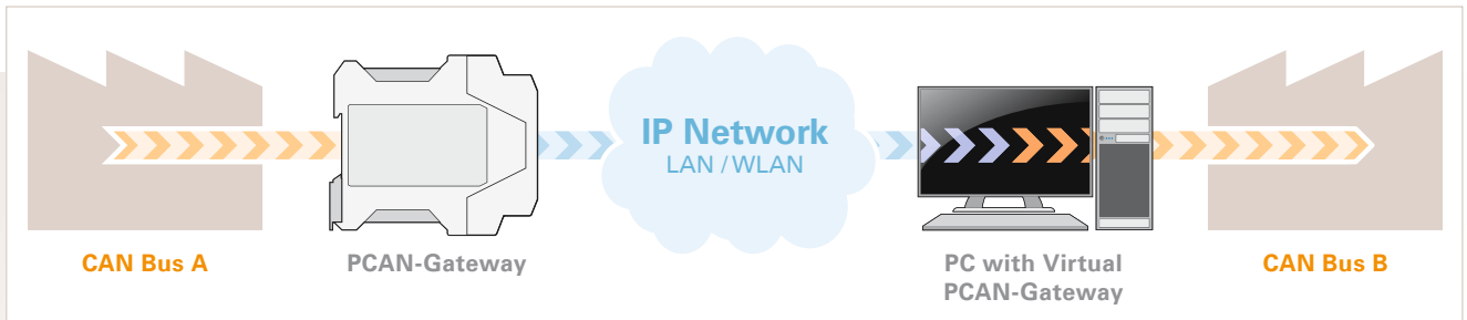
Example 4: Connection via the software Virtual PCAN-Gateway
