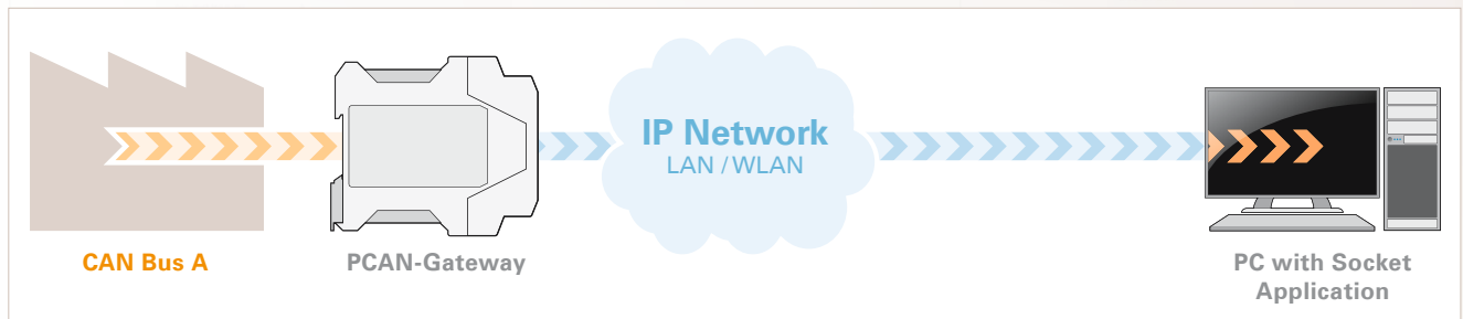
Example 3: Connection via a Socket Application
